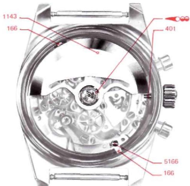
45. Grease the friction between the center wheel (206) and the cannon pinion (245)(00»»)and sette cannon pinion.
