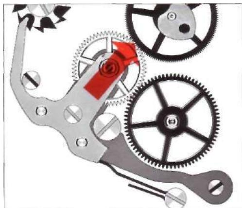
If so, delicately separate the coupling clutch so as to provoke disengaging between the coupling wheel and the chronograph wheel.
