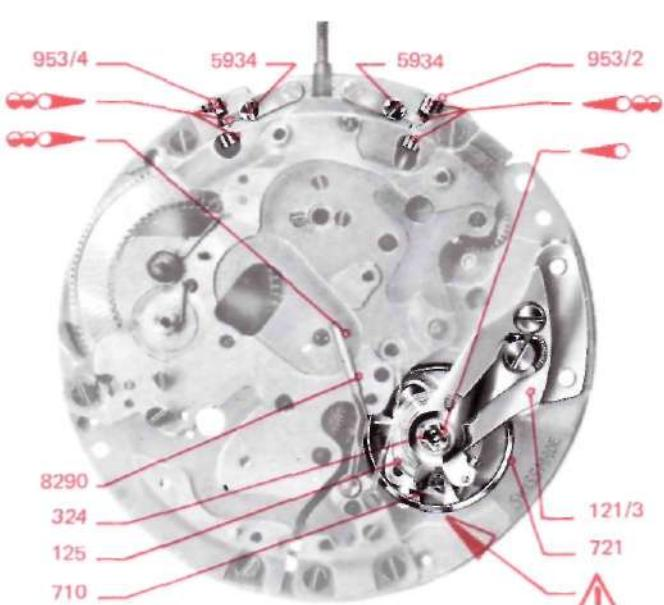
7. Grease the pivot of the winding stem fixed in the plate (CC^->) the pivoting point of the detent (443) and lower setting wheel (450).
