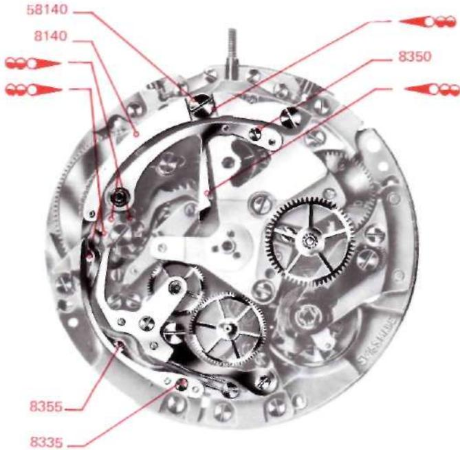
19. Set the blocking lever (8200), grease ( e©c^-) and fasten its screw. Check that the shortest part of the blocking lever spring (8345) is between the pivoting center and the lower pin of the blocking lever.
